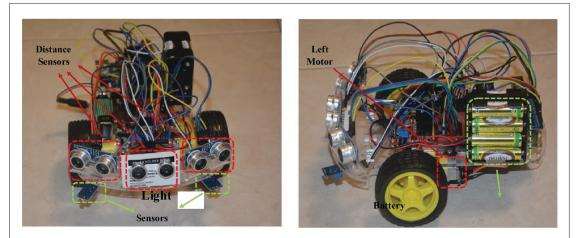
Figure 2. A typical robot developed by students in COMP 5228 course in Fall 2016. The read-made chassis is equipped with batteries, light sensors, distance sensors and micro-controller board. The chassis has two driving wheels and a supporting free wheel. A video (made by student) showing basic functions of the robot is available online at: https://www.youtube.com/watch?v=opnJ1zlHvSA.
